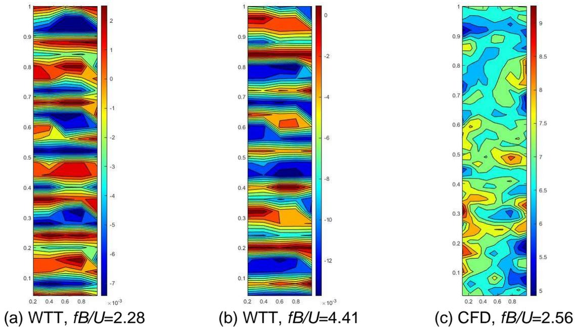
Fig. 4 DMD mode shape at the local peak on high frequency
