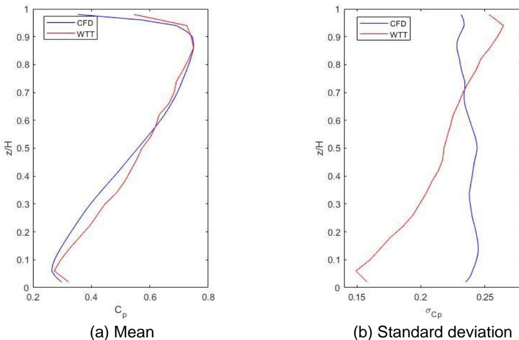
Fig. 2 Wind pressure coefficient on windward wall
